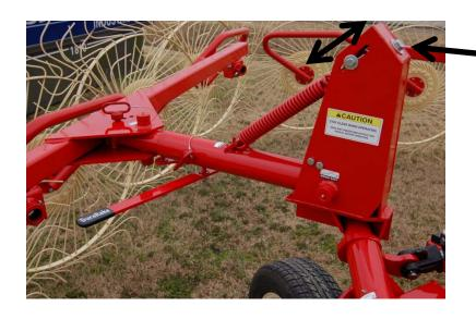
Tighten bolt for less ground pressure and loosen bolt for more ground pressure. When correctly adjusted the tines on all of the rake wheels should be deflected the same when the rake is in operation. If they are not you will need to add more ground pressure. For the rake to perform properly the rake wheels must have enough ground pressure for the tines to be deflected where they contact the ground while raking.
